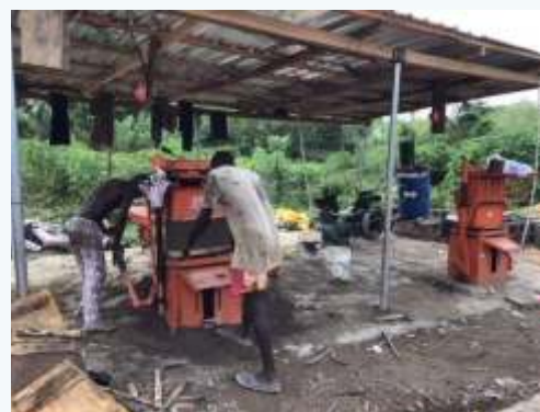
Operators of the block molding machine at the ACE Cooperative Society block industry
